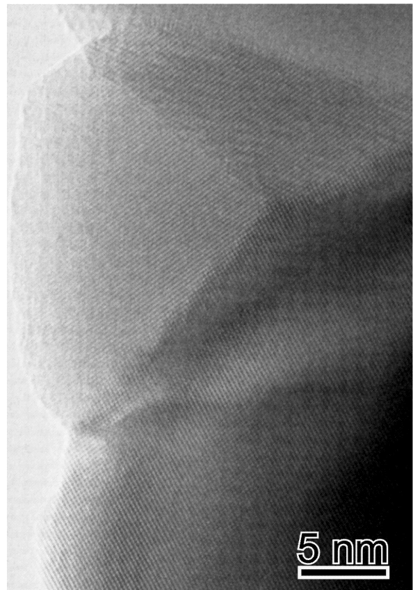
Fig.10 A lattice image of a part of the ZnO nano-chain.
