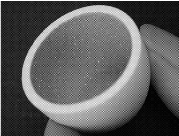
Fig.2 Alumina crucible coated with ruby crystal films.
