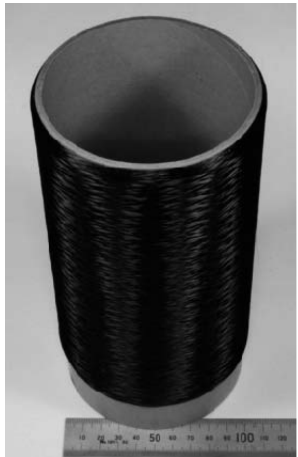
Fig.3 SiC fibers designated by Nippon Carbon Co., Ltd. (NICALON, Type NLM-102).
